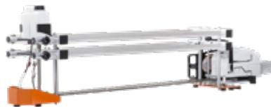
The saw frame stabilizes the guide bar. On the top of the saw frame there are functions such as, water cooling and separate oil pump for effective lubrication of the chain. On the chainsaw side there is a saw carriage with a crank for comfortable and even feeding forward.
